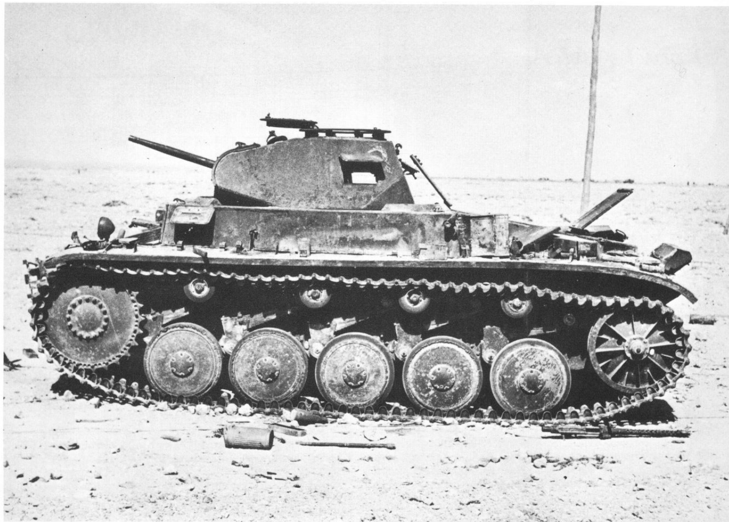
A burnt out PzKpfw II Ausf A-C photographed after the fighting around Sollum at the end of April 1941 shows up well the profile view of the type after it had been fitted with a turret cupola. Note the MG34 co-axial gun lying on the ground under the rear idler, and its barrel near the centre roadwheel.
