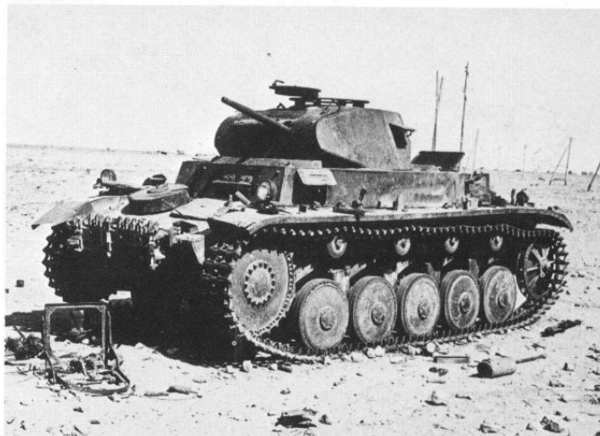
Another view of the burnt out vehicle. Note the spare tracks added to the nose to enhance protection. This photograph was taken on the 2nd of May, 1941.
