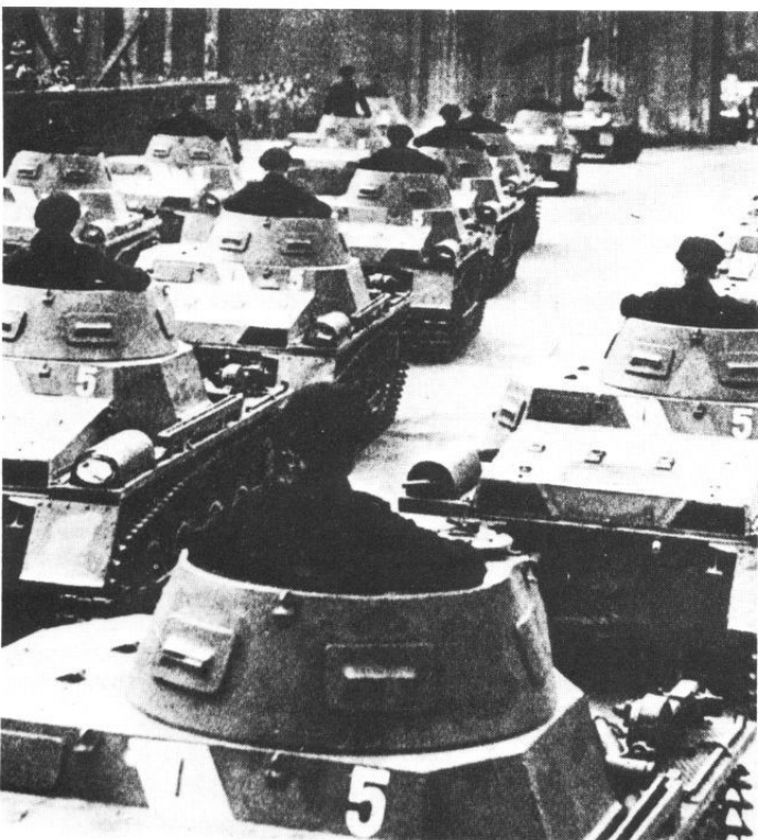
Parade of early production PzKpfw I Ausf. A in Berlin, pre-war. Note the rear decks have no oil cooler or air outlet armoured cover.
